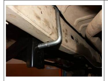
Place three U-bolts around the passenger side chassis rail so that they roughly line up with the feet of the side steps.
