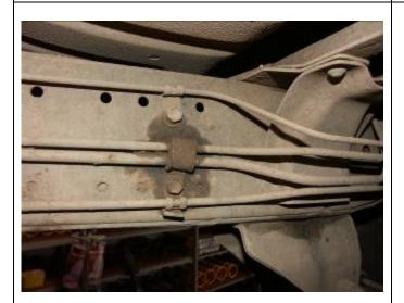
On the driver's side chassis rail, undo the brake and fuel line retaining bolts and place the U-Bolts between the chassis rail and the fuel and brake lines.
